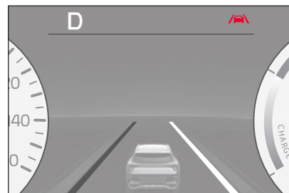
When LKA detects the vehicle moving outside of the lane being traveled in, a yellow lane marker will illuminate either on the left or right lane (shown in both images above)
