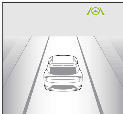
When the front-view camera does not detect the lane markers, they are displayed gray
